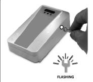
Adjust the Half Flush cycle time by holding the Magnetic Wand against the right side Magnetic Target until the desired water release is achieved. Note the speed and distance of the Flush Motor up/ down cycle and adjust accordingly. The Full Flush cycle will be set automatically in relation to the Half Flush cycle.
